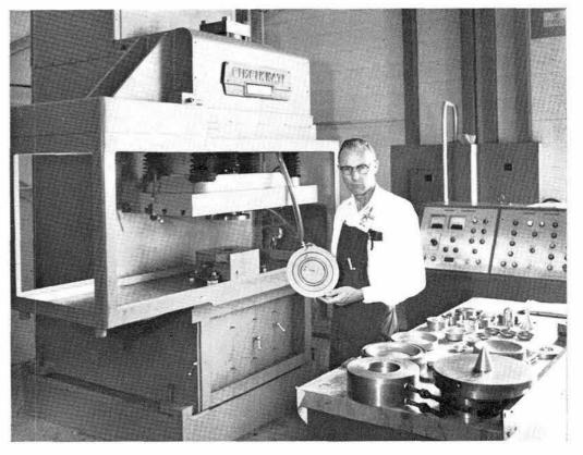
RAPID FORMING is done with this Electroshape which transforms electrical energy into mechanical motion. The hydroelectric effect enables the Sheet Metal Section 4232-5 to make formed parts in as little as 0.0004 seconds.
